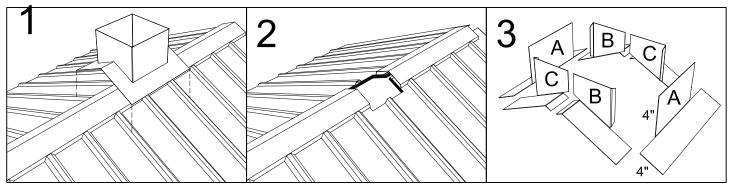
Place ridge flashing over existing metal roof and trace using the inside of the duct as template.
