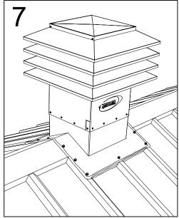
Install ventilator head over the ridge flashing, making sure it is level and fasten with screws provided into each of the perforated holes. (Model 301 shown)
