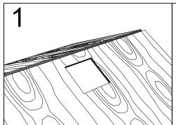
Cut out opening in roof deck to reflect the same size opening of the slope flashing to be installed.
