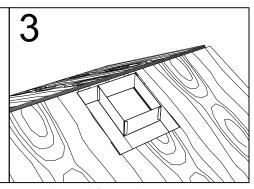
Assemble and fasten the counter flashing onto roof deck around the perimeter of the opening.
