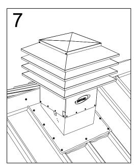
Install ridge cap over flashing. Place ventilator head over the slope flashing, making sure it is level and fasten with screws provided into each of the perforated holes. (Model 301 shown)
