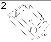
Fabricate a galvanized metal counter flashing (4" high x 4" flange) as illustrated above, supplied by contractor.
