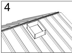
Install metal roof over the counter flashing as illustrated above and then seal around all joints with bitumen tape or caulking.
