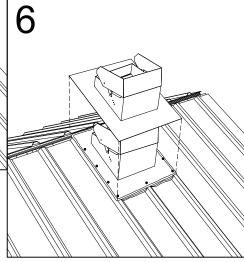
Install slope flashing over the counter flashing and fasten onto metal roof and deck (screws supplied by contractor). Install a quality bitumen sealant around the perimeter of the flashing, filling up all gaps between metal and flashing.
