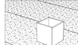
Install the curb centered on the opening and fasten it to the roof using screws. (fasteners supplied by the contractor)
