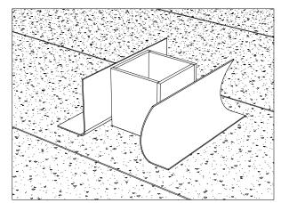
Waterproof the curb by installing a membrane on all its horizontal and vertical surfaces. Follow the installation instructions recommended by the membrane manufacturer.
