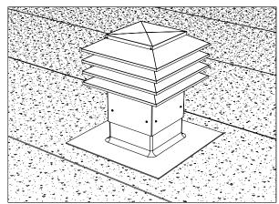
Install the head of the ventilator on its flashing by fastening it using the supplied self-tapping screws. Make sure to install the screws at a minimum height of 203mm (8') from the finished roof system.
