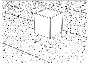
Build a wooden curb to fit inside the vent with the proper allowance for the membrane and place the curb on the roof at the desired location. Make sure the opening is located between structural beams. Trace a line on the roof from inside the curb.
