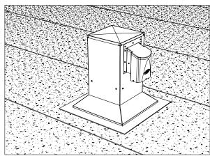
Install the head of the CT-AD-12 on its flashing by fastening it to the flashing using the supplied self-tapping screws. Make sure to install the screws at a minimum height of 203mm (8') from the finished roof system.
