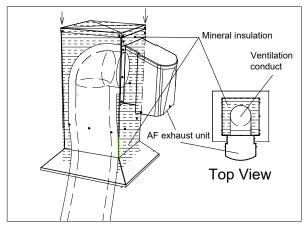
Fill-in the remaining space around the duct with mineral insulation and re-install the cover of the CT-AD-12, making sure of tightening all screws.
