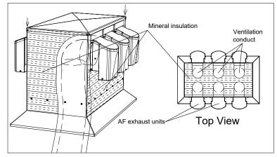
Fill-in the remaining space around the duct with mineral insulation and re-install the cover of the CTM, making sure of tightening all screws.
