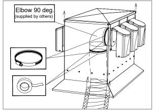
Remove the top cover of the CTM and install an 90deg elbow of the right size over the collar of the AF traps, using an adjustable collar. Secondly, install a duct (flexible 2in insulated duct is recommendeded) around the 90 deg. elbow using an adjustable collar. Seal all connections using a good quality duct tape.
