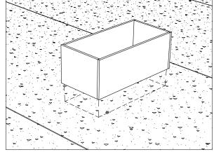
Build a wooden curb to fit inside the vent with the proper allowance for the membrane and place the curb on the roof at the desired location. Make sure the opening is located between the structural beams. Draw a line on the roof from inside the curb.
