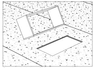
Cut an opening in the roof following your traced line. Apply an amount of bitumen under and along the perimeter of the
