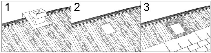
Place flashing over desired area making sure it is positioned between the rafters. Using the inside duct as a template, trace a line around the inside perimeter onto the deck. Opening should start 6-8 inches down from ridge.
