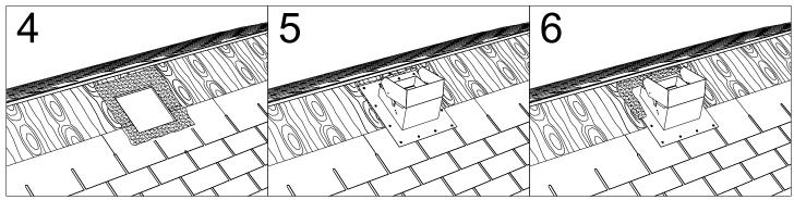
apply a generous amount of bitumen cement over the top portion of the shingle parallel with the hole as illustrated.
